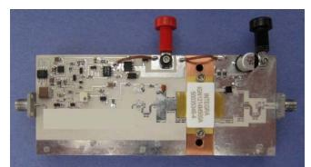
Figure 1: IGN1214M500 Amplifier with bias sequencing and gate pulsing circuitry
